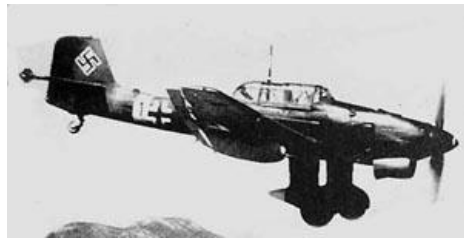
Junkers JU 87 "Stuka" Seats: 2 County of Origin: Nazi Germany Maximum Speed: 180mph Range: 465 Miles Armament: 4x.31 (front & rear), External bombload
