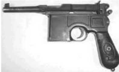
Mauser C-96 "Broomhandle" Caliber: 7.65mm (also in 9mm) Shots: 10 Country of Origin: Germany Year first made: 1896
