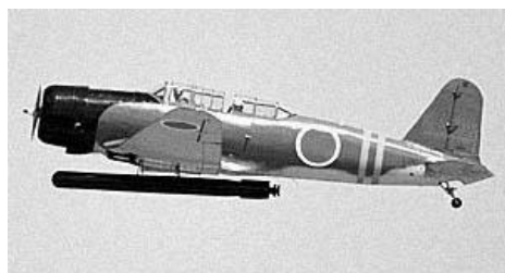
Nakajima B5N2 "Kate" Seats: 3 County of Origin: Japan Maximum Speed: 235mph Range: 1,237 Miles Armament: 1x.30 cal machine gun (rear), 1x1,764 lb torpedo or bomb weight equivalent
