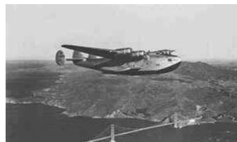
Boeing B-314 Seats: 74 Cruising Speed: 183mph Maximum Speed: 193mph Range: 3500 Miles
