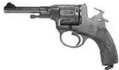
Nagant gaz-seal revolver Caliber: 7.65mm Shots: 7 Country of Origin: Belgium Year first made: 1892
