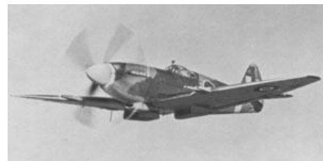
Supermarine Spitfire Seats: 1 County of Origin: Great Britain Maximum Speed: 378mph Range: 1140 Miles Armament: 2 x 20mm cannons, 4 x .303 Browning machine guns
