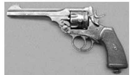
Webley Revolver Caliber: .455 Shots: 6 Country of Origin: Britain Year first made: 1887
