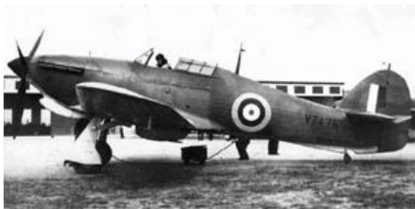
Hawker Hurricane Mk I Seats: 1 Maximum Speed: 330 mph Range: 460 Miles Armament: 8 Browning .303 Machineguns
