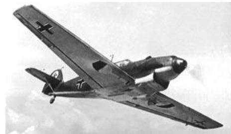
Messerschmitt Bf 109 Seats: 1 County of Origin: Nazi Germany Maximum Speed: 398mph Range: 528 Miles Armament: 2x13mm machine guns, 1x 20mm cannon, 4x 110 lb bombs
