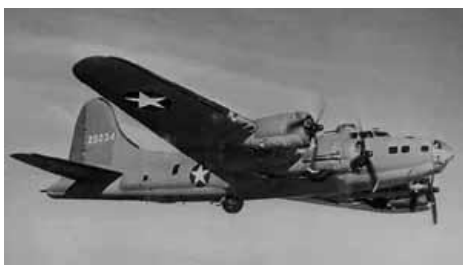
B-17 "Flying Fortress" Seats: 10 Maximum Speed: 287mph Range: 2000 Miles Armament: 9x.50 Cal Machineguns, 4,000-pound bomb load, 10x 5in Rockets
